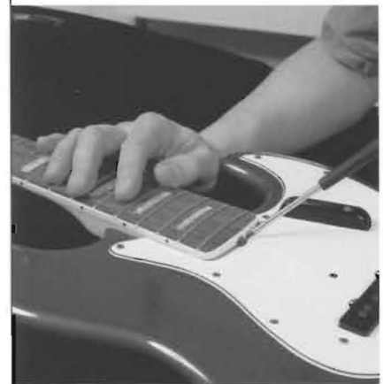
The truss-rod adjuster is at the end of the neck. Make sure you use the correct tool. (Here the screwdriver is only being used as a pointer to illustrate the location of the adjuster.)
